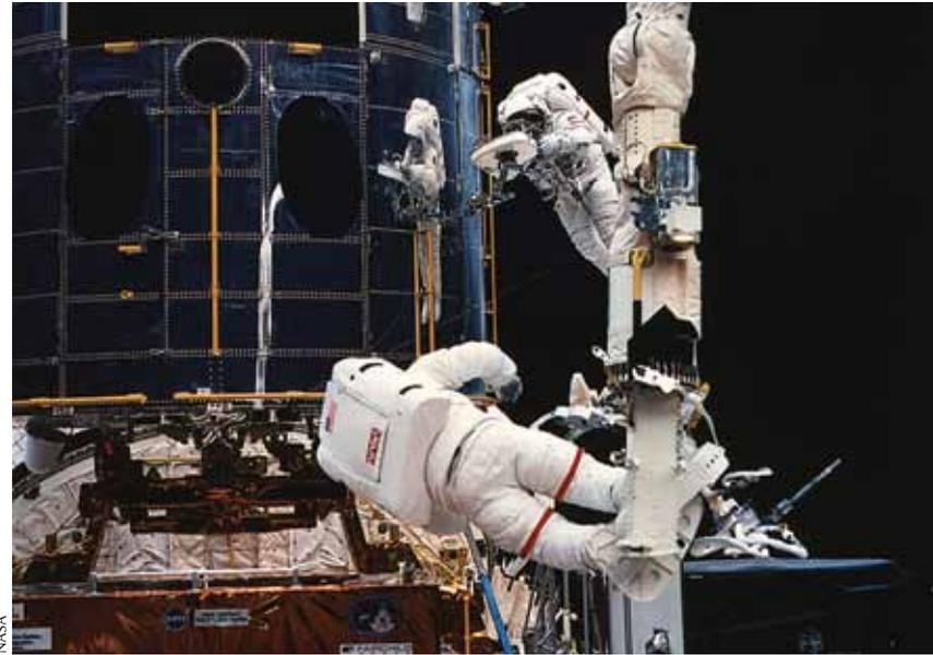
Anchored on the end of orbiter Endeavour's remote manipulator system arm, astronaut Jeffrey Hoffman (foreground) prepares to install the new wide field planetary camera into the empty cavity of the Hubble Space Telescope (HST). Astronaut Story Musgrave works with a portable foot restraint.
